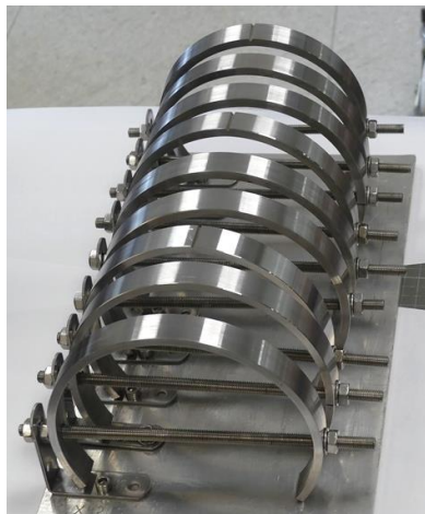
Rack with tested C-ring specimens
