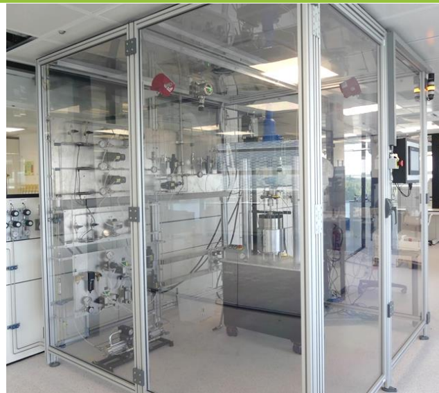
SSRT tensile, fracture and fatigue machine for testing in H 2 gas in Tecnalia H2Lab
