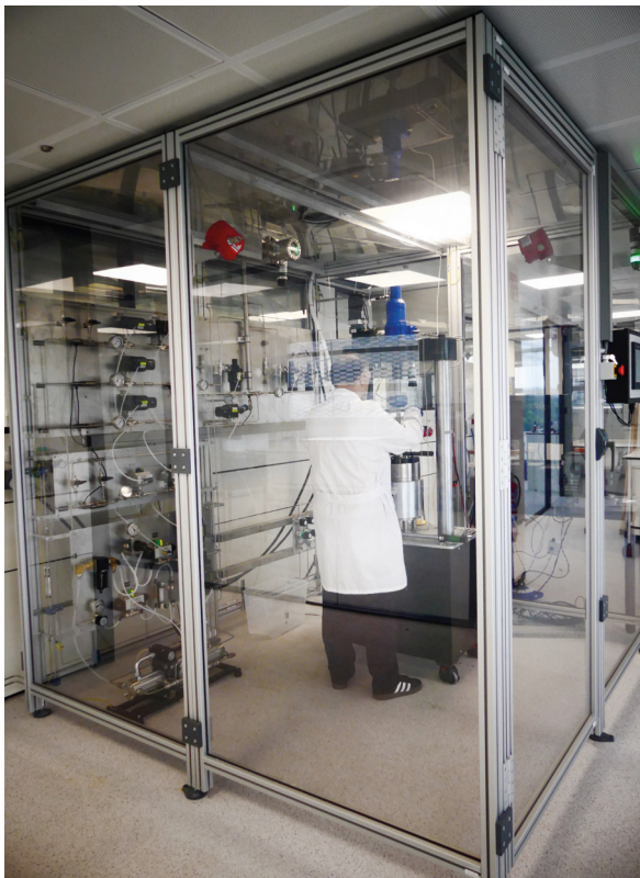
Figure 4: SSRT tensile, fracture and fatigue machine for testing in \text{H}_2 gas
