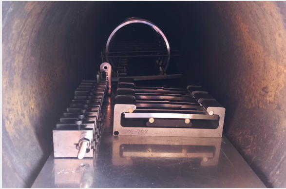
Figure 3: Insertion of strained specimens in the pig trap
