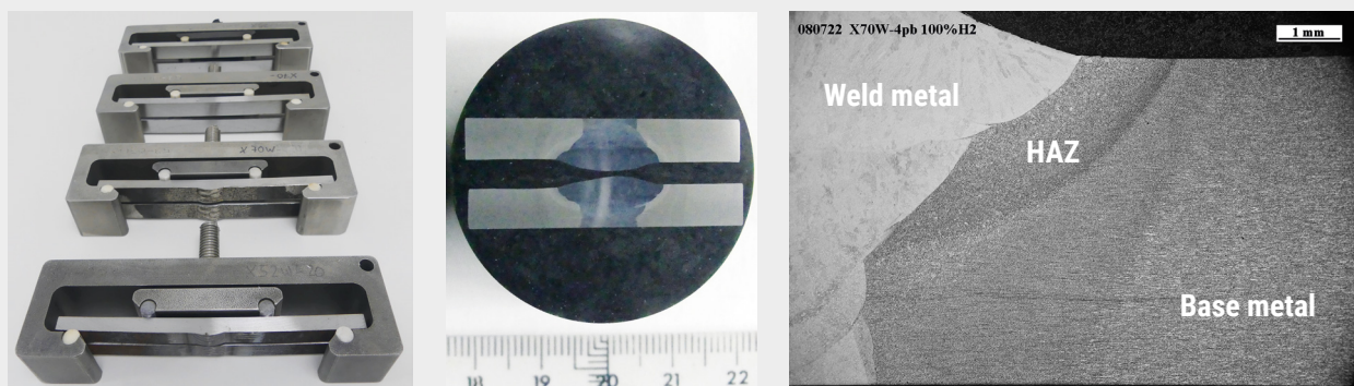
Figure 8: 4pb specimens after the 100% hydrogen campaign (left); detail of embedded cross sections (center); optical micrograph of X70 welded 4pb cross sections after the 100% hydrogen campaign (right)
