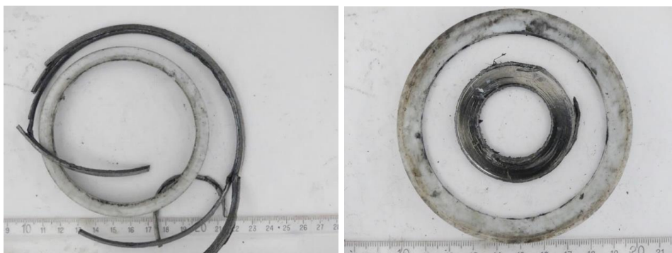
Figure 21. Detail of teflon and graphoil seals in flanged ball valve C-V-15 (left) and C-V-16 (right)
