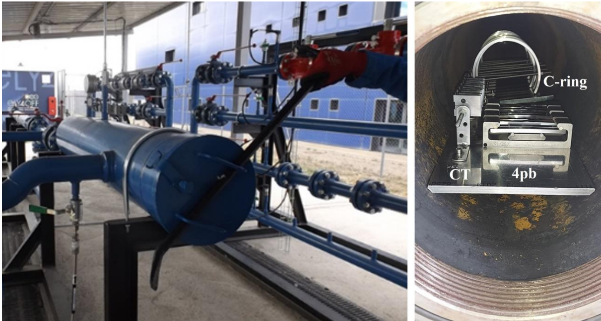
Figure 3. Picture of the pig trap (left) and the constant strain specimens allocated inside it (right)
