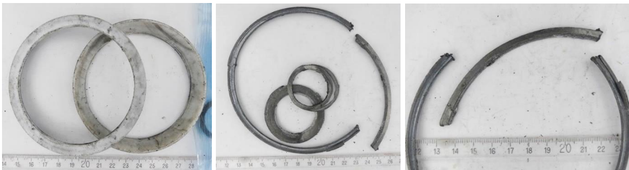
Figure 20. Flanged ball valve C-V-17. Detail of teflon seals (left) and graphoil body seals (center and right)
