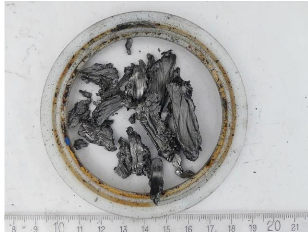
Figure 22. Detail of teflon and graphoil seals in DIDTEK butterfly valve seal
