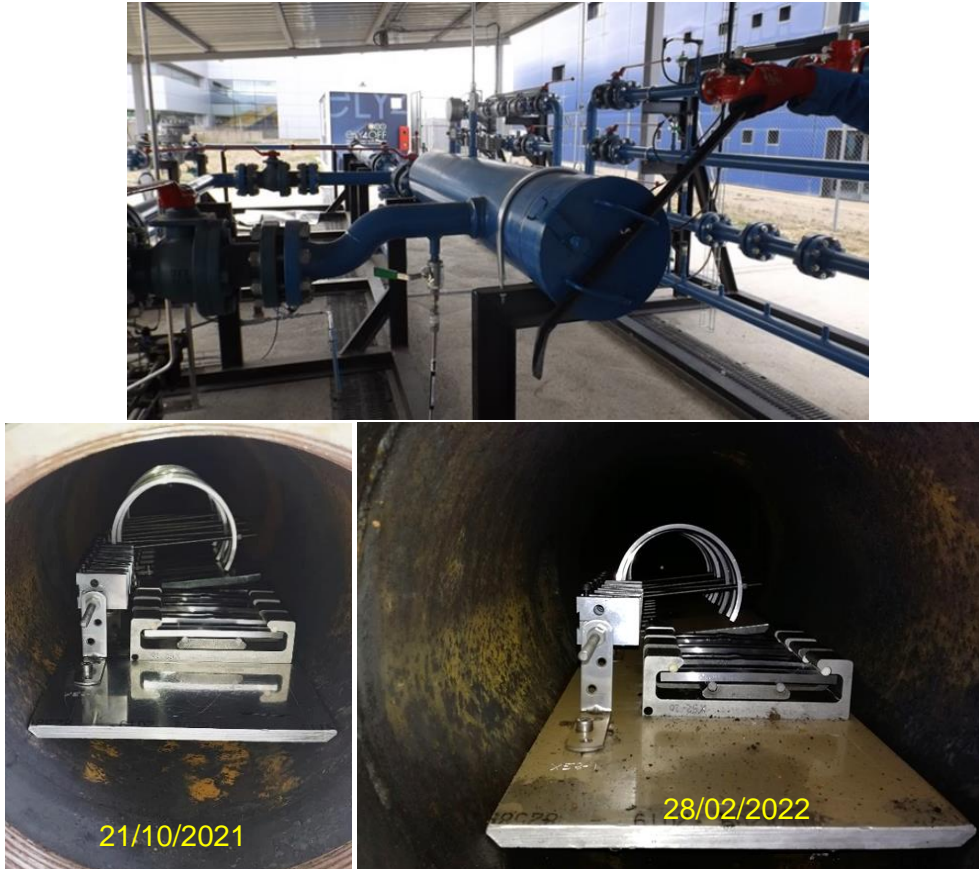
Figure 5. Test specimens inside the pig trap in the loop experimental platform at FHA at the beginning of the test, and once concluded
