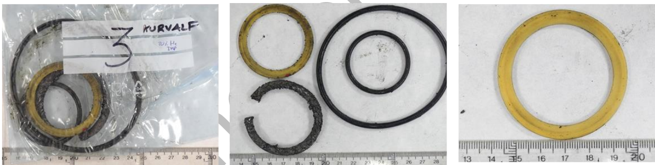
Figure 9. Components of the KURVALF plug valve (left) showing detail of the O-rings (middle) and the graphoil and Teflon seals (right)
