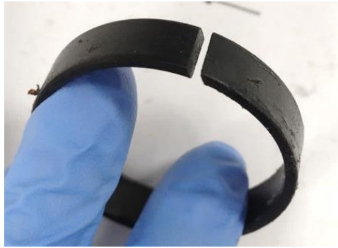
Figure 4. Pilot guide ring from the pressure regulator
