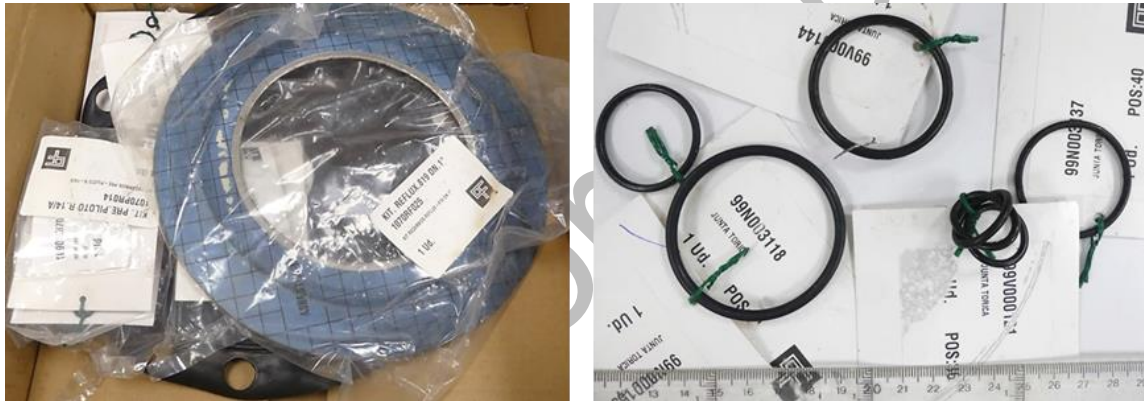
Figure 2. Parts of the pressure regulator (left) and detail of some of the pilot O-rings inspected (right)
