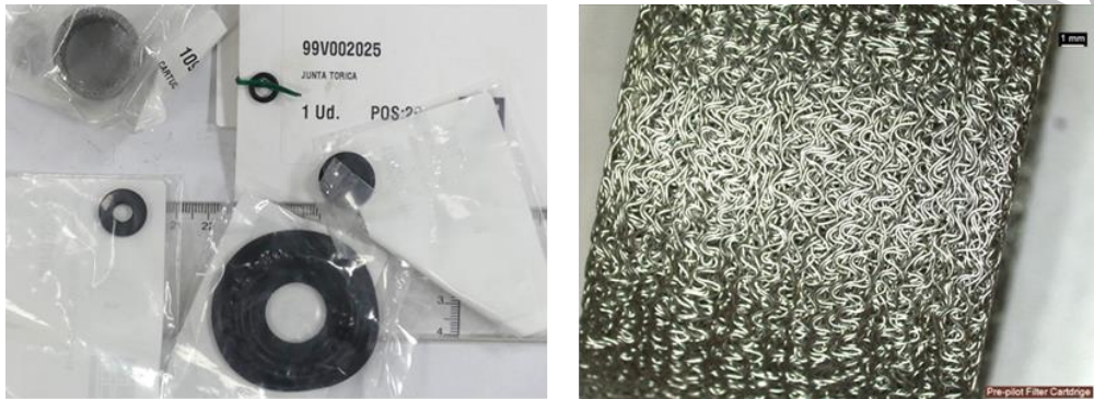
Figure 5. Pre-pilot pressure regulator components (left) and detail of filter cartridge (right)
