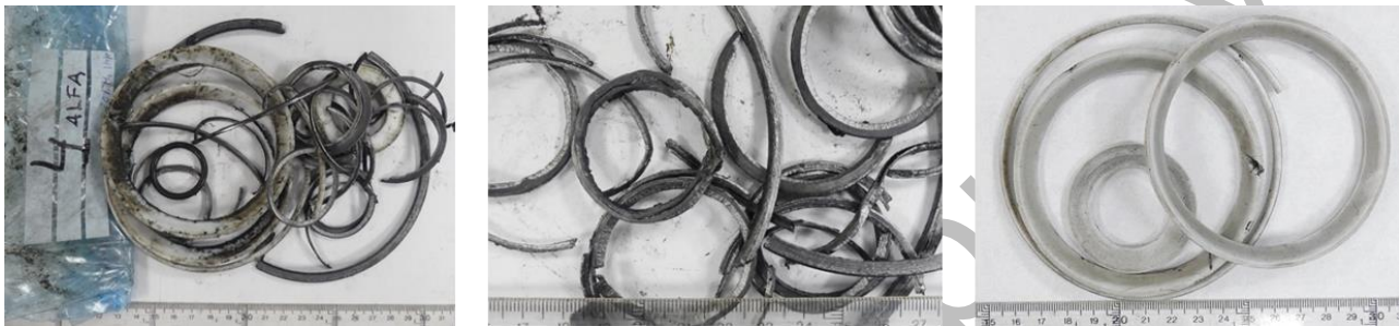
Figure 8. Components of the ALFA VALVOLE ball valve (n° 4) (left) showing detail of the graphoil (centre) and Teflon seals (right)
