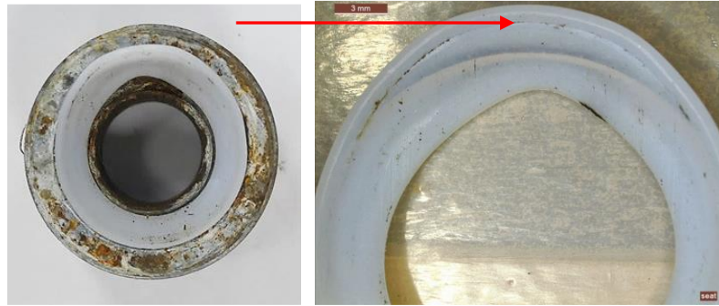
Figure 12. Photographs showing detail of the deformed TFM seat
