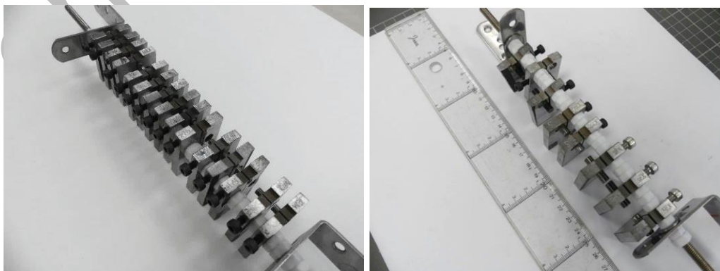
Figure 21. Rack with tested CT bolt loaded specimens in the 2 nd campaign (left) and in the 3 rd campaign (right)
