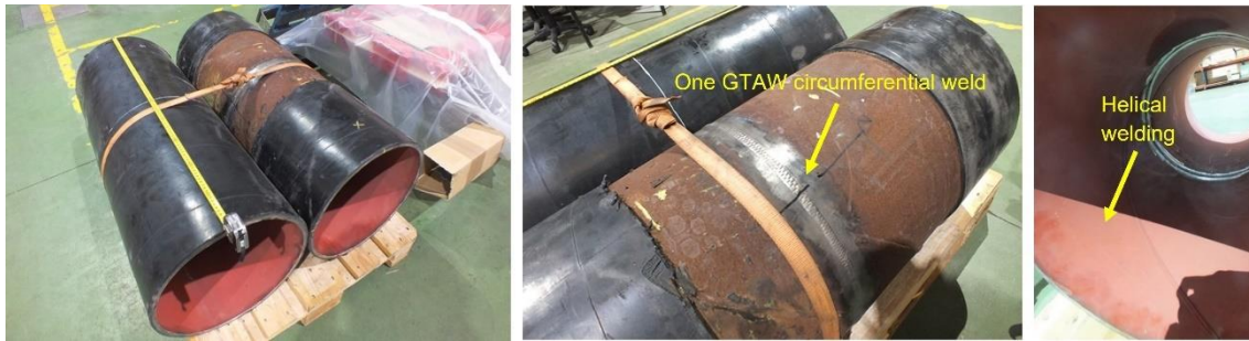
Figure S3. Photographs showing detail of the two sections of the X70 steel pipe as example
