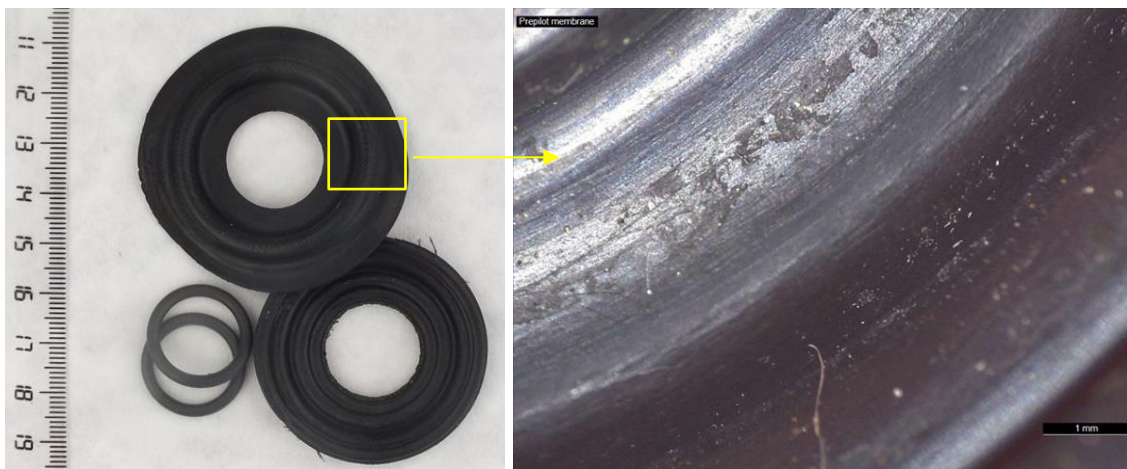
Figure S10. Pilot: membranes and guided rings (left) and detail of eroded area (right)
