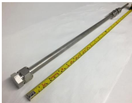
Thin Pd-based supported membrane (up to 5 \mu\text{m} thick)
