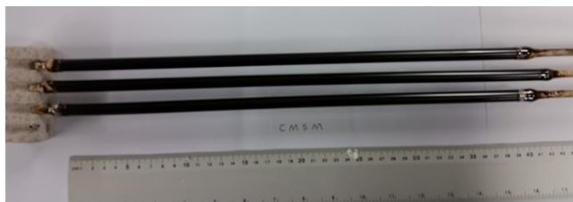
Thin carbon molecular sieve membrane (~3 \mu\text{m} thick)
